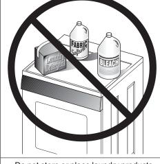
Do not store or place laundry products on top of dryer at any time. They can damage the finish or controls. **WARNING** To reduce risk of fire or serious injury to persons or property, comply with the basic warnings listed in *Important Safety Instructions* and those listed below.
